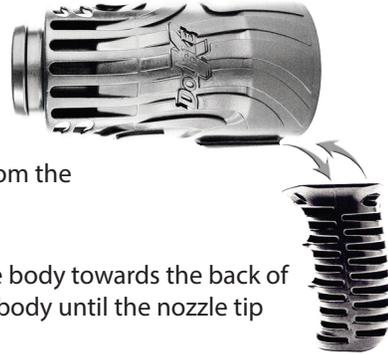
**Attaching nozzle tips:** Place the front of the nozzle body towards the back of the nozzle tip. "Rock" the nozzle tip onto the nozzle body until the nozzle tip locks into place. Check if it is secure by gently pulling the nozzle tip and nozzle body.
