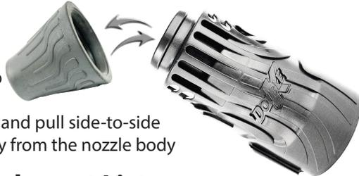
**To remove a nozzle tip:** Firmly grasp the nozzle body with one hand and the tip with the other. "Rock" or push and pull side-to-side while pulling the tip in a motion away from the nozzle body until the tip is released.
